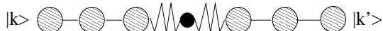
FIG. 1: Schematic representation of a system composed of two semi-infinite current/voltage leads and a scattering region, where inelastic scattering can occur. An electron with k -vector k approaching the scattering region from the left is transmitted to the right with k -vector k' . In this 1D case if k \neq k' the energy is not conserved.
