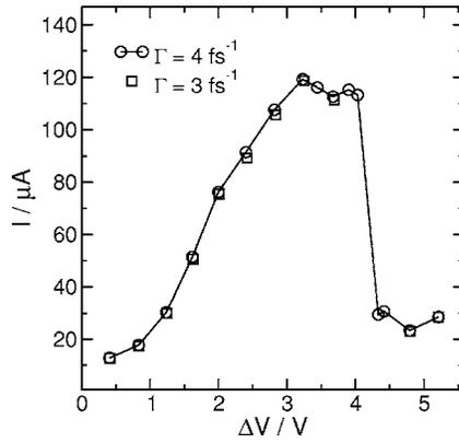
FIG. 3. Current-voltage curve obtained from the final values of the current and potential difference after a steady state has been reached, for two different values of the parameter  $\Gamma$ .
