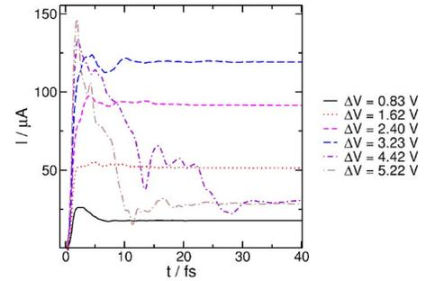
FIG. 2. Current as a function of time from the integration of Eq. (2). The bias shown corresponds to the final steady state.
